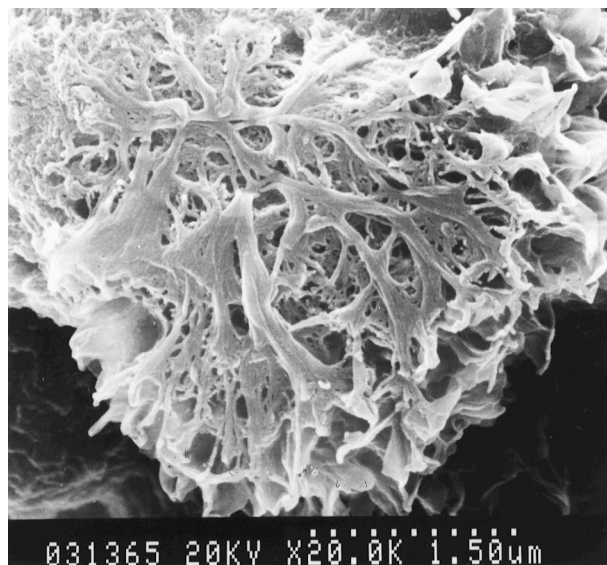
Fig. 8. SEM photomicrograph of a PVDF crystallite. Dope: point E in Fig. 2.
